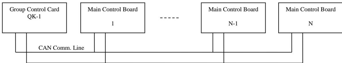
**Remove** the terminal resistors R287 & R252 (which resistor has marking 620, i.e. 62 ohm) near to J4 of Main control boards from board 1 to board N-1.
