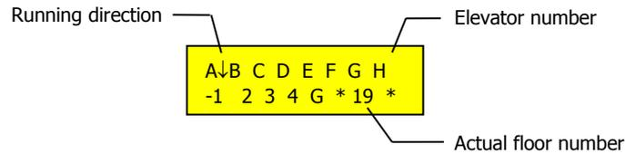
A, B, C, D, E, F, G and H are representing the eight elevator numbers; the arrow beside it is indicating the elevator running direction; the number or alphabet below the elevator number is showing the current actual floor number; if a symbol “\*” is under the elevator number, it means there is communication abnormal or “Group able set” is set to “NO” (or it may be set to Mode:0 in that elevator main control board Group control function)
